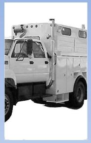
A truck which is able to transport a crew to the jobsite. This truck has multiple seats in the cab and has multiple seats in the modified bed. The truck carries compartments for the crew's tools and supplies. Some tools this vehicle may carry are compressors, generators, ladders, and many other important tools and supplies.
