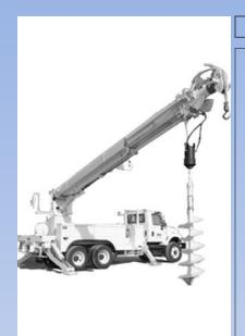
A type of truck mounted lifting arm, or boom, with an auger attachment. It is designed to accommodate such tasks as digging holes, setting poles, and maneuvering material. An auger can come in various diameters and lengths, and attaches to the side of the boom.
