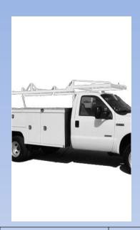
A truck which assist the crew by carrying most of the tools and supplies. It has multiple compartments to carry everything necessary to complete a job. Some tools and supplies this vehicle may carry are compressors, generators, ladders, and many other important tools and parts.
