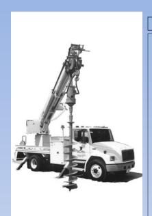
A type of truck mounted lifting arm, or boom, with an auger attachment. It is designed to accommodate such tasks as digging holes, setting poles, and maneuvering material. An auger can come in various diameters and lengths, and attaches to the side of the boom.
