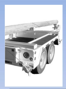
A trailer which is able to carry one or multiple poles at different lengths. The pole carrying assembly includes rail bolsters (supports) with adjustable pole cradles. The trailer also comes with a center pole saddle on the extendable trailer tongue. All pole trailers also come with multiple load tie downs. Most of these trailers are able to connect to a standard tow hitch ball mounted at the rear of a tow vehicle.
