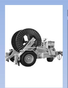
A trailer with one or multiple revolving turret reels for hauling spools of wire/cable. Each type of trailer is capable of carrying a certain payload. Some are single axel and some are tandem. Some turrets can be turned by hand and some use motors. Many are also cable pullers or tensioners, which means that they are capable of assisting with installing and removing of cable. Most of these trailers are able to connect to a standard hitch ball mounted at the rear of a tow vehicle.
