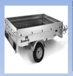
A flat bed trailer which carries extra tools and supplies for the crew. Some tools and supplies this vehicle may carry are compressors, generators, and many other important tools and parts.
