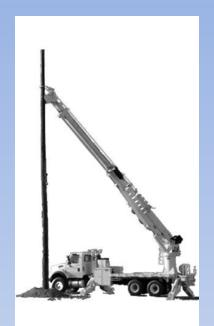
A type of truck mounted lifting arm, or boom, with an auger attachment. It is designed to accommodate such tasks as digging holes, setting poles, and maneuvering material. An auger can come in various diameters and lengths, and attaches to the side of the boom.
